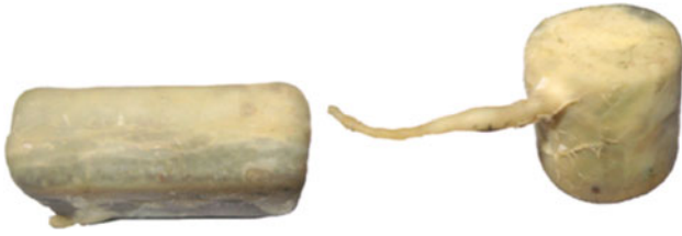
Fig. 5 The parts after being coated by national rubber in outer surfaces
